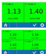
Vib-Eye adapts the layout of the home page to optimize the view of the installed sensors: 2,4,8 CUBEs can be displayed simultaneously.
